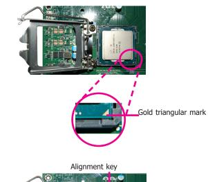
The CPU's notch will prop-erly fit into the socket's alignment key.
