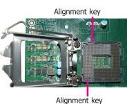
8. Close the load plate then push the load lever down.
