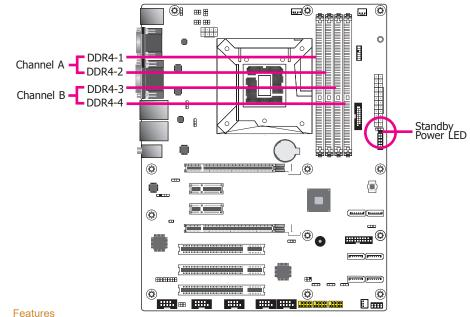
The four DIMM sockets are divided into 2 channels:
